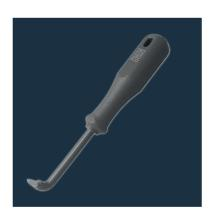
Special tool for easy removal of cover caps from assembled lever handle sets. Suitable for round roses, oval roses, and short and long plates. Steel zinc-plated, blade width 4 mm, with protective black nylon sheath.
