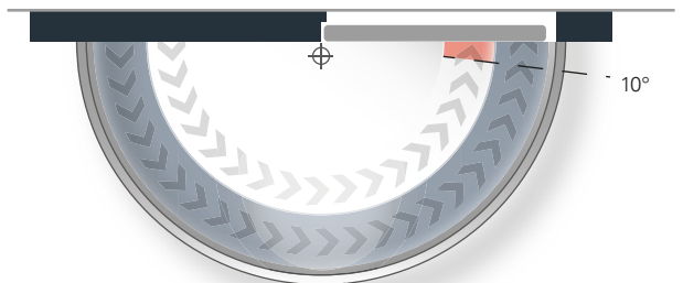
Closing force diagram ECO Newton TS-14 EN, hinge side
