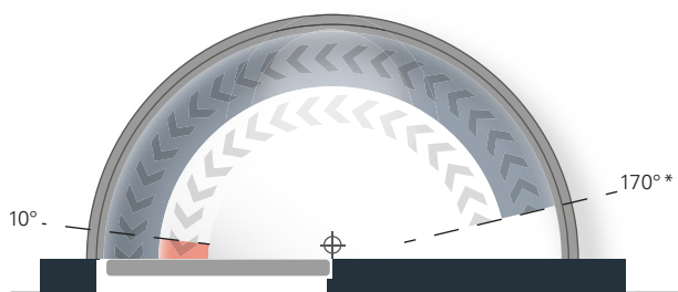
Closing force diagram ECO Newton TS-14 EN, opposite hinge side
